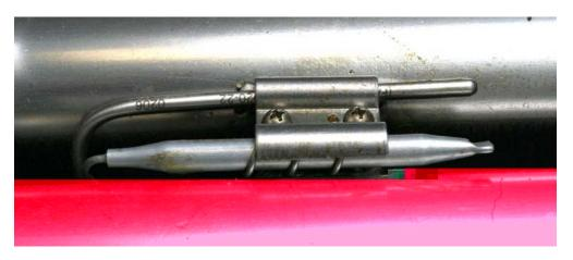
Typical high-limit/sensor probe locations and mounting hardware.
